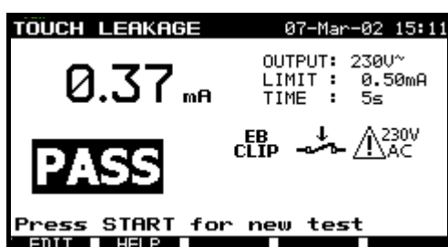
Fig. 4.41 Good result example of touch leakage test
