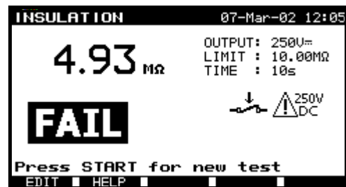
Fig. 4.18 Bad result of insulation test
