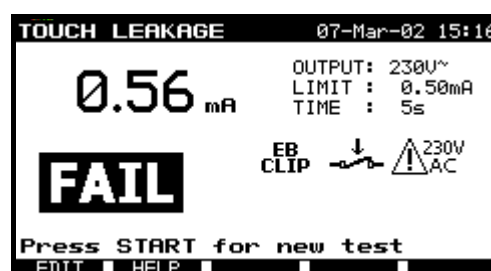
Fig. 4.42 Bad result example of touch leakage test
