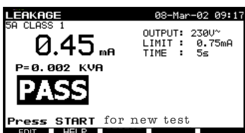
Fig. 4.35 Good result example for leakage current and power test
