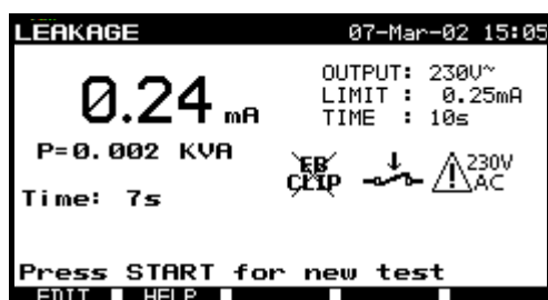
Fig. 4.37 Display of aborted leakage current and power test
