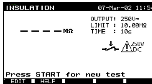
Fig. 4.16 Insulation test initial display
