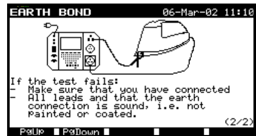
Fig. 4.4 Help for reasons of failed earth bond test
