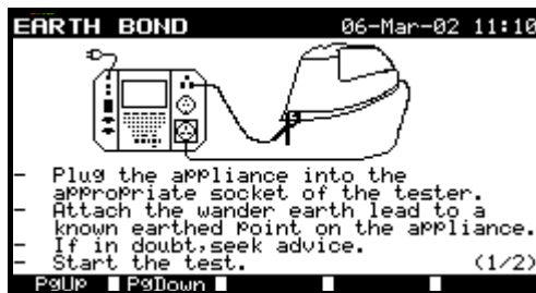
Fig. 4.3 Help example for earth bond test connection
