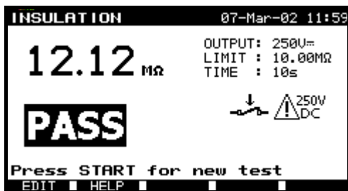
Fig. 4.17 Good result of insulation test
