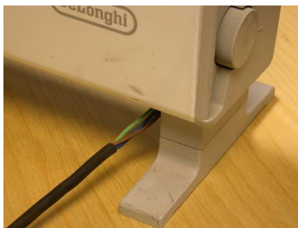
Cable not being gripped.
