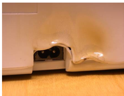
Damage to external casing.
