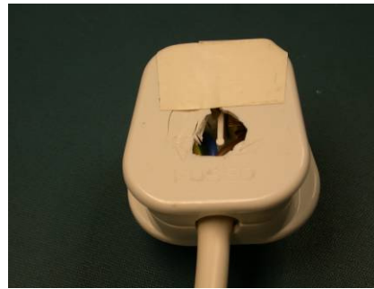
Damage to mains plug.
