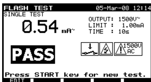
Examples of flash test results
