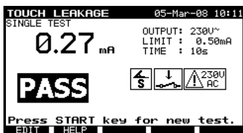
Examples of touch leakage current measurement results
