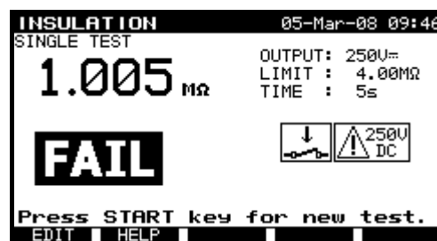
Examples of insulation resistance measurement results
