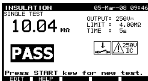
Examples of insulation resistance measurement results
