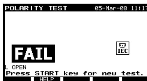
Examples of polarity test results
