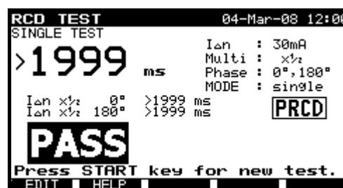
Examples of RCD single test results
