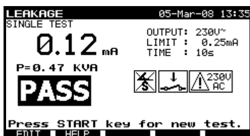
Examples of leakage current and apparent power measurement results
