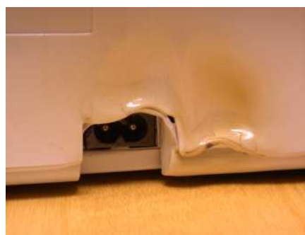
Damage to external casing.
