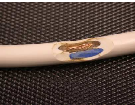
Damage to power cable sheath.
