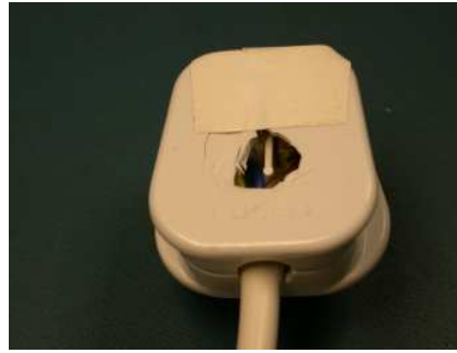
Damage to mains plug
