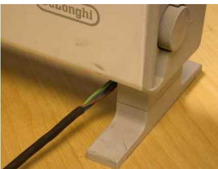
Cable not being gripped.
